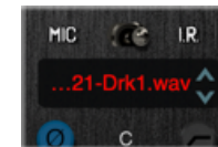
Missing IR indicated by red text in Channel Strip IR menu
